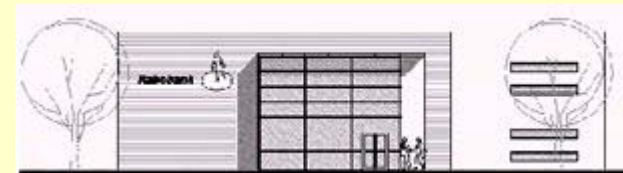
Netherlands: Office building Rabobank, Zierikzee The design team focussed on minimising the HVAC-system by an adequately designed building envelope. This resulted in a design with an estimated reduction of energy consumption of about 30%.
